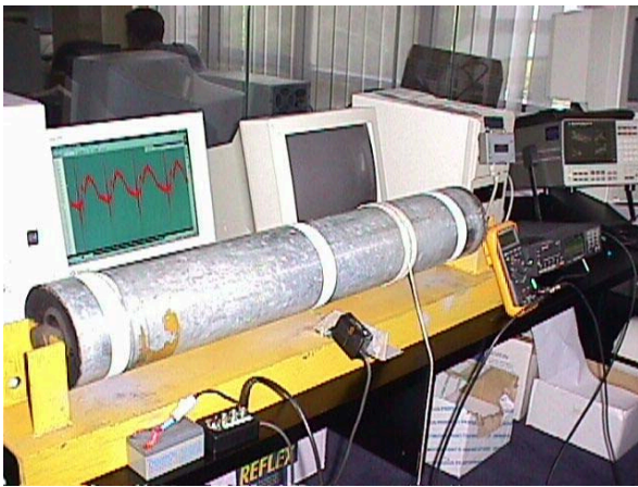
Figure 5. Photograph of Surface Profile Measurement Set Up
