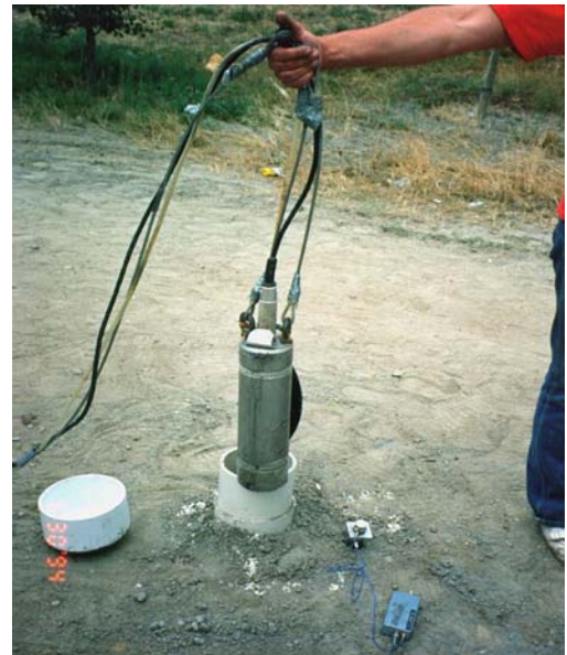
Figure 1 Groundborne noise and vibration survey borehole and measurement equipment
