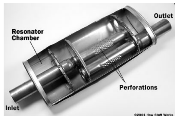
Figure 1: Typical reactive automotive muffler
