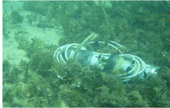
Figure 2. Photo of acoustic logger, located in predominantly Amphibolis antarctica off Guichenault Point, Shark Bay
