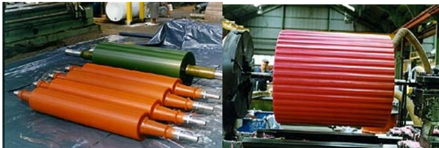
Figure 2 Typical Conveyor Rolls Lined with Polyurethane Coatings
