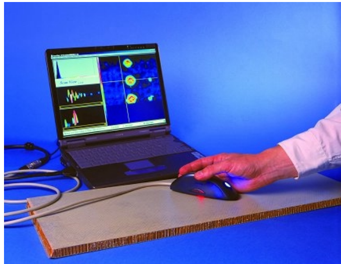
Figure 5 - The Bandicoot demonstrator system examining a Nomex cored test panel.
