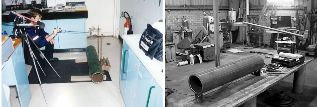
Figure 3 Impact Test Trials 1999-2000 for Polyurethane coated rolls
