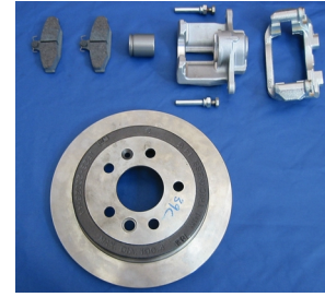
Figure 2: Brake system individual parts: (clockwise from top left) pads, piston, pins, caliper housing, anchor bracket and rotor
