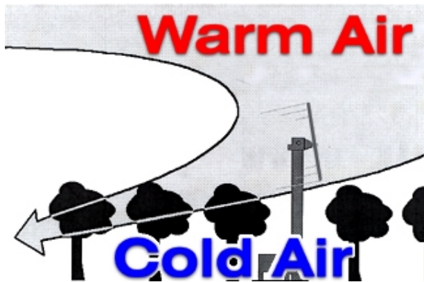
Figure 2. The Wind Machine Principle. (Courtesy of the Amarillo Wind Machine Company, USA) [1].
