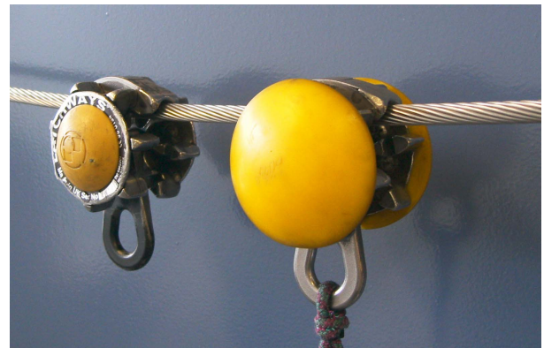
Figure 5. Pictures of Original (left) and Modified (right) Latches.
