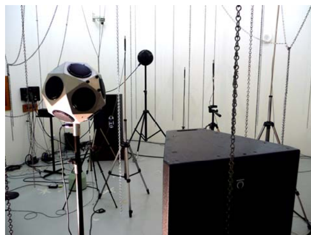
Figure 3. Microphone and loudspeakers set up in the reverberant room
