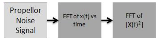
Figure 5 Schematic of cyclostationary propeller detection process
