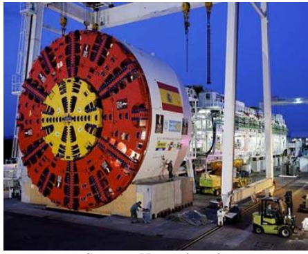
Source: Herrenknecht Figure 2. Herrenknecht (EPB) TBM
