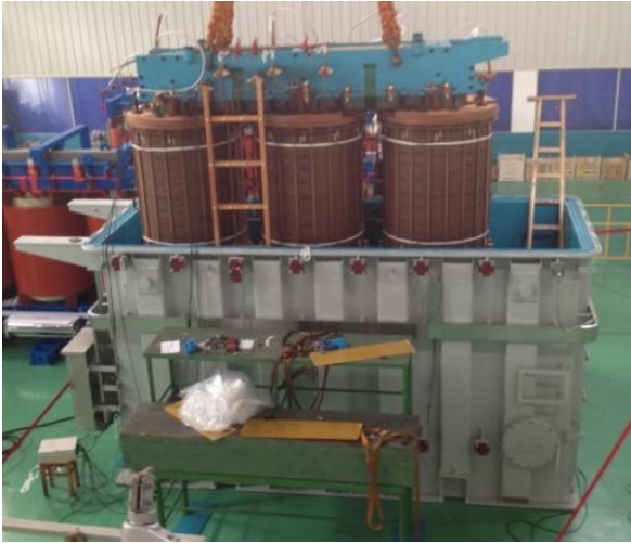
Figure 1: The tested transformer before assembly*. (*All the tests were implemented after assembly.)
