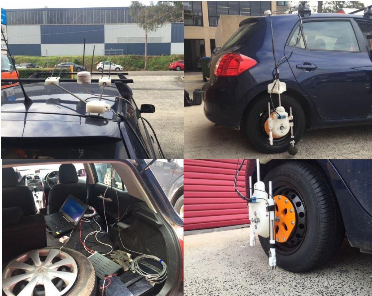
Figure 4. Images of a test vehicle fitted with the SLR OBSI system
