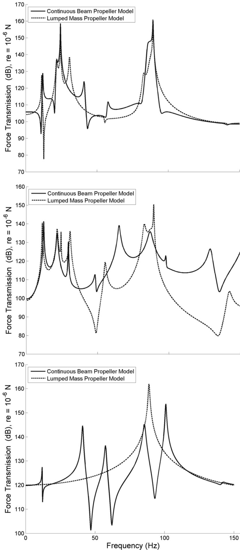
Figure 3. Force transmission through the journal bearing (top), thrust bearing (middle) in the  $y$  directions and force transmission through the thrust bearing in the  $z$  direction (bottom)
