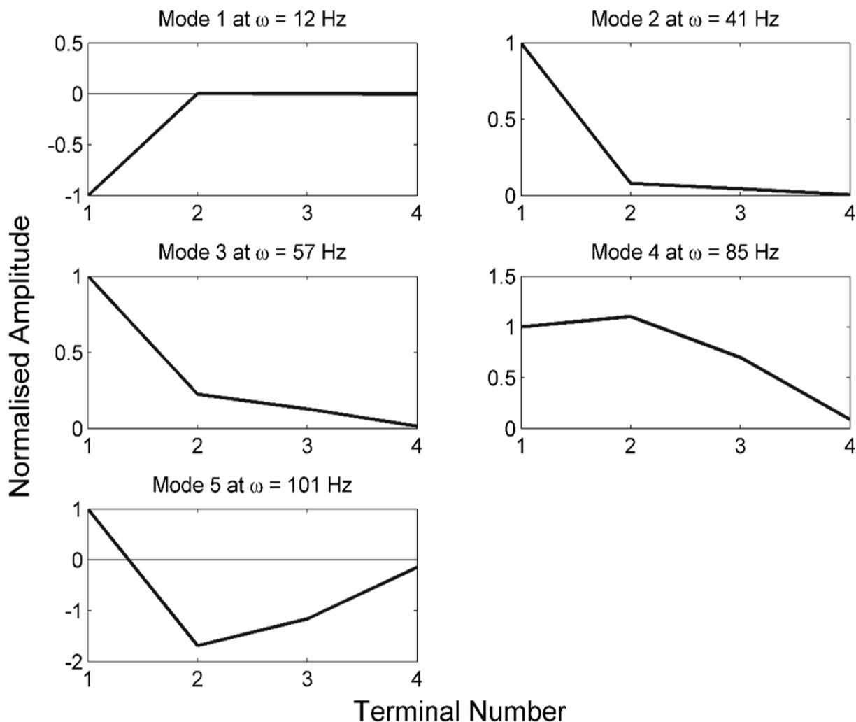
Figure 4. Axial vibration mode shapes
