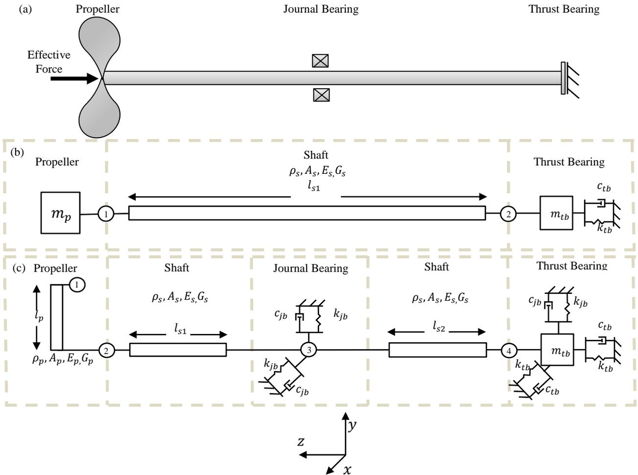
Figure 1. Top: (a) Diagram of system. Middle: (b) Schematic of propeller shafting system of previous studies. Bottom: (c) Schematic of propeller shafting system in this study and its coordinate system
