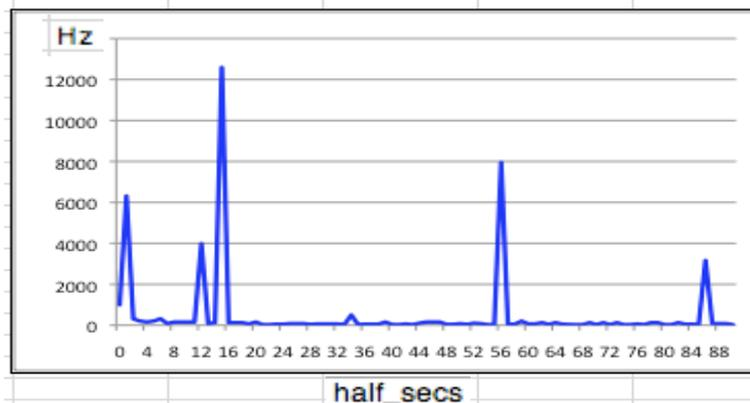
Fig. 16 Shows the dominant third-octave frequency as a function of time ‘Dominant’ is meant in the sense of the level at the centre frequency of the filter that exhibits the maximum protrusions above the levels of its immediate neighbours (“pitch” discrimination).
