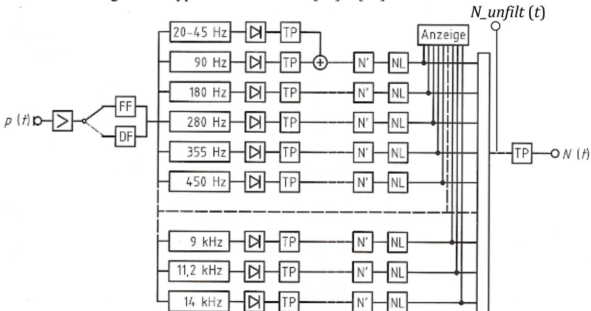
Fig.1 Schematic of the dynamic loudness algorithm (DIN 45631/A1)
