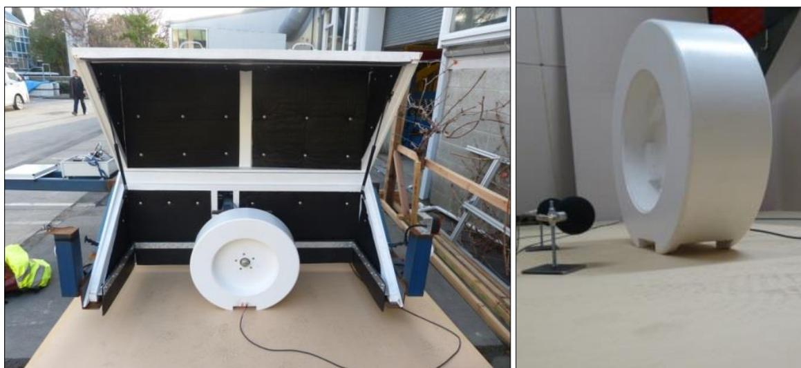
Figure 3. Artificial sound source inside and outside a CPX trailer (University of Canterbury)
