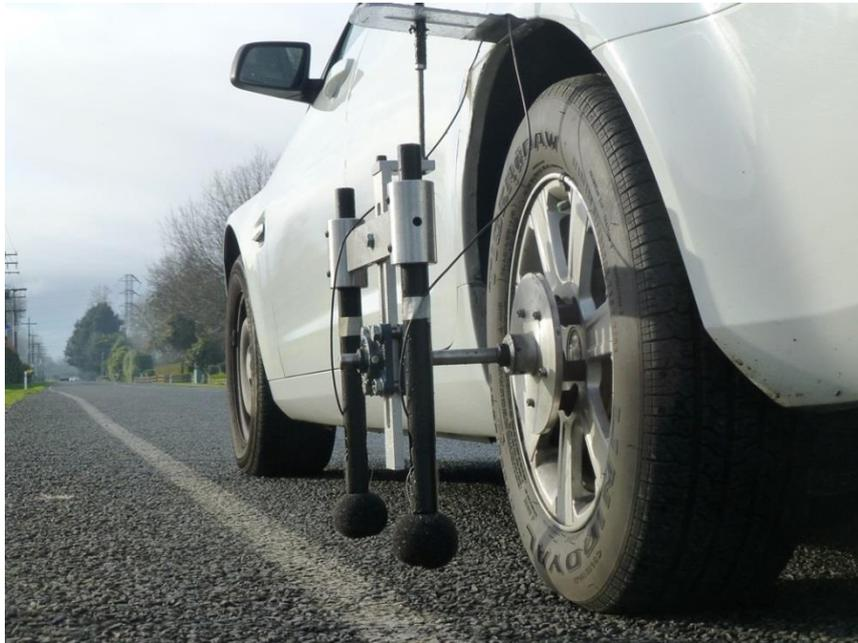
Figure 1. Microphone bracket fitted to the rear wheel of a test vehicle (Opus Research)
