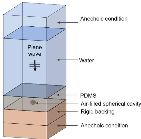
Figure 1: Schematic diagram of a unit cell of the acoustic coating.
