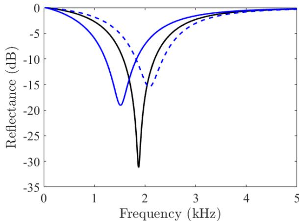
Figure 8: Reflectance (in dB) of the acoustic coating for the original sized voided inclusion in the absence of hydrostatic pressure (black line), for the same coating under hydrostatic pressure of 0.7 MPa (blue line), and of a coating without hydrostatic pressure but with a reduced size void (dashed blue line).
