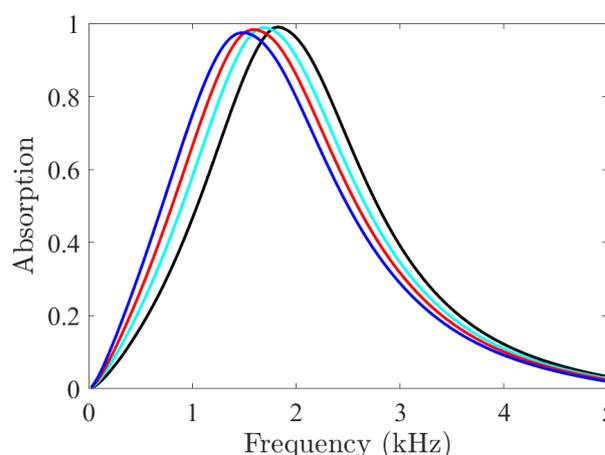
Figure 7: Absorption coefficient of the acoustic coating in the absence of hydrostatic pressure (black line) and under hydrostatic pressure of 0.3 MPa (cyan line), 0.5 MPa (red line) and 0.7 MPa (blue line).
