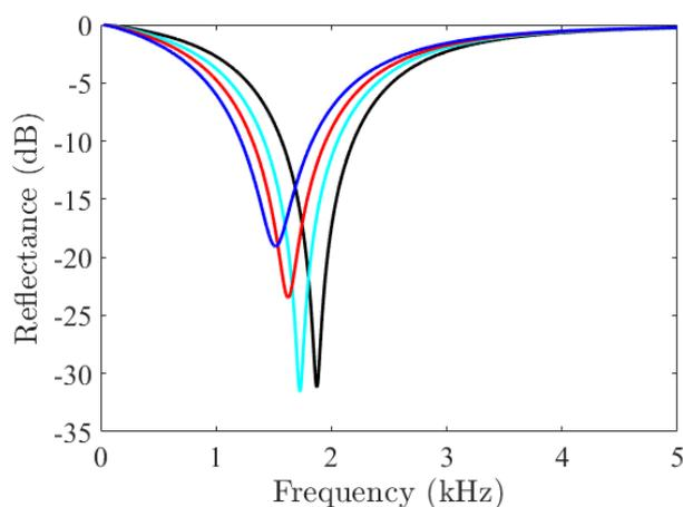
Figure 6: Reflectance (in dB) of the acoustic coating in the absence of hydrostatic pressure (black line) and under hydrostatic pressure of 0.3 MPa (cyan line), 0.5 MPa (red line) and 0.7 MPa (blue line).
