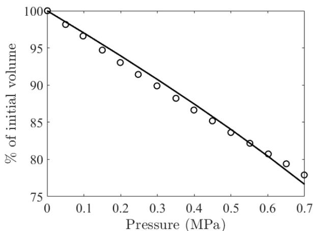
Figure 2: Percentage reduction in inclusion volume arising from an increase in hydrostatic pressure obtained numerically (solid line) and from Thieury et al. (2019) (circles).
