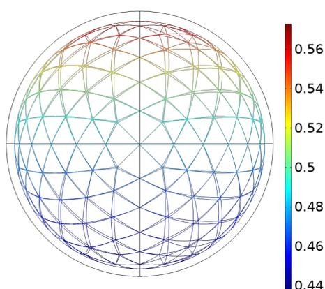
Figure 4: Deformation (in mm) of the inclusion resulting from uniaxial compression of the PDMS at a hydrostatic pressure of 0.3 MPa. The undeformed geometry is represented by the black circle.
