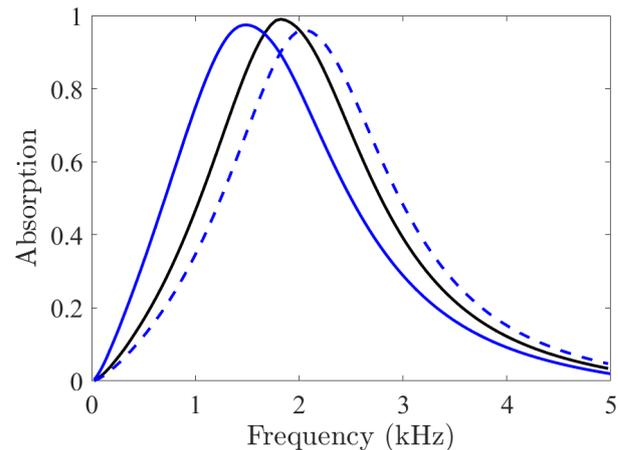
Figure 9: Absorption coefficient of the acoustic coating for the original sized voided inclusion in the absence of hydrostatic pressure (black line), for the same coating under hydrostatic pressure of 0.7 MPa (blue line), and of a coating without hydrostatic pressure but with a reduced size void (dashed blue line).
