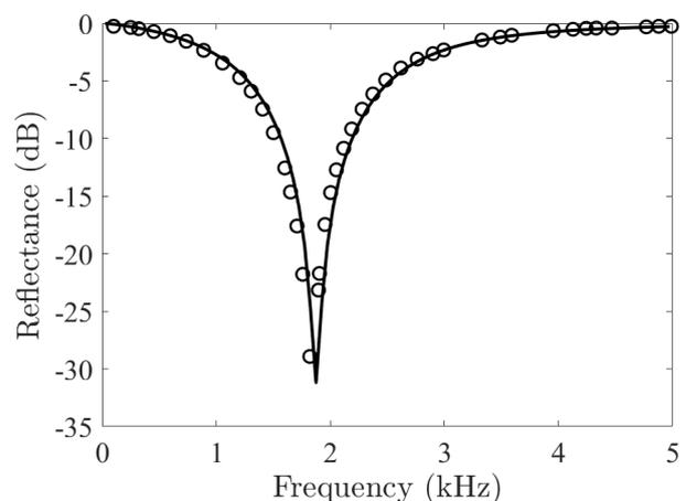
Figure 3: Reflectance (in dB) of the acoustic coating in the absence of hydrostatic pressure obtained numerically (solid line) and from Thieury et al. (2019) (circles).
