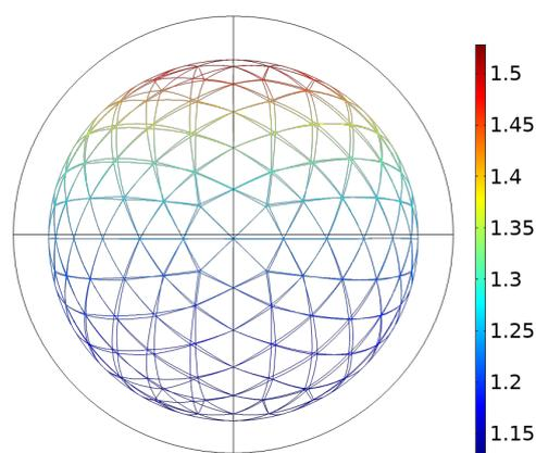
Figure 5: Deformation (in mm) of the inclusion resulting from uniaxial compression of the PDMS at a hydrostatic pressure of 0.7 MPa. The undeformed geometry is represented by the black circle.
