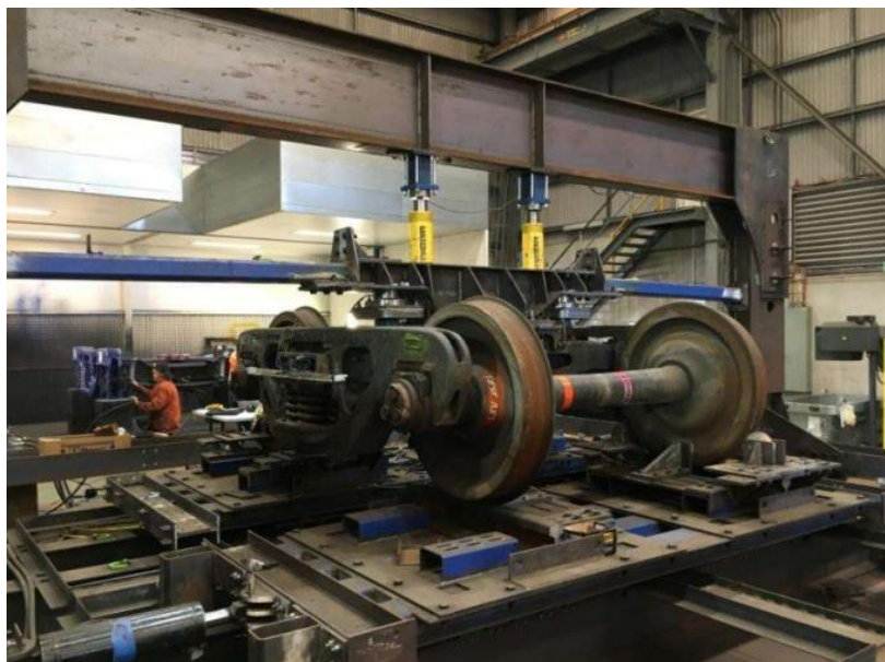
Figure 4 TfNSW bogie test rig (Jiang, 2018)
