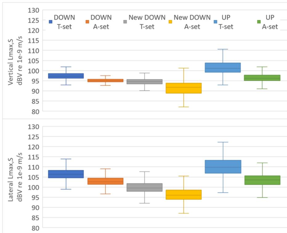
Figure 4: Vibration mean and quartile distribution by axis, track and train type. Outlier results not shown.
