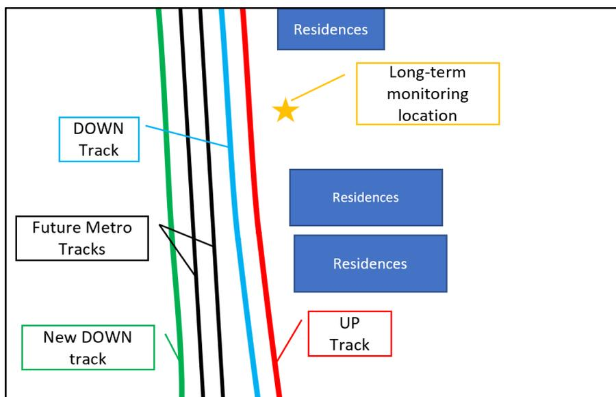
Figure 1: Monitoring location and track configuration. DOWN track relocated to new location in March 2021.
