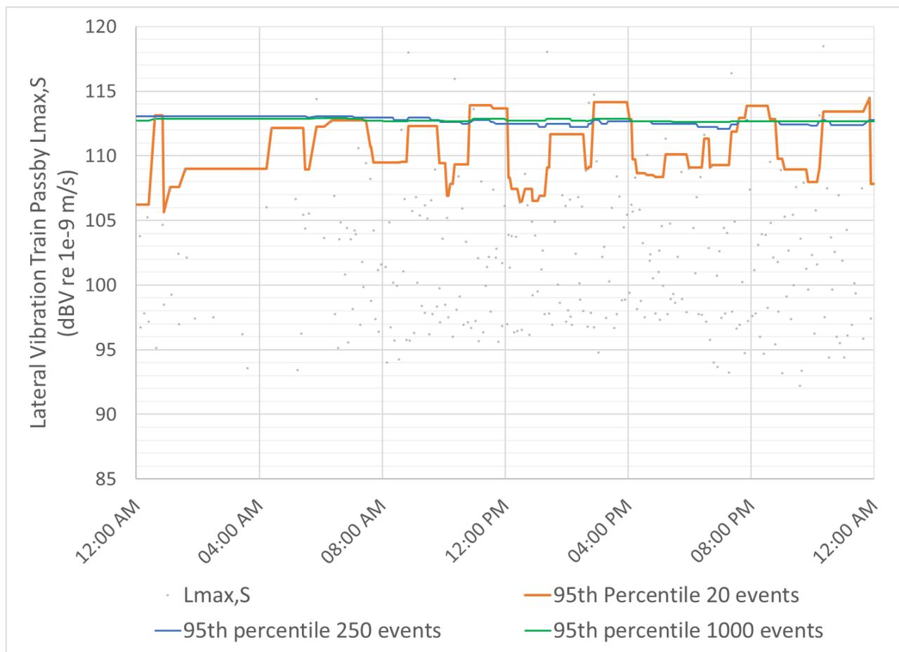
Figure 6: One day example (April 26<sup>th</sup> 2021) showing variability in 95<sup>th</sup> percentile vibration level from 20 events
