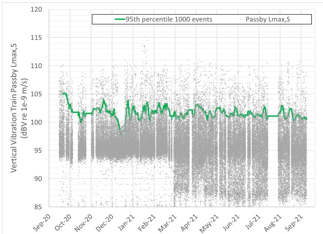
Figure 3: Vertical train passby vibration dataset with individual events and 95<sup>th</sup> percentile levels
