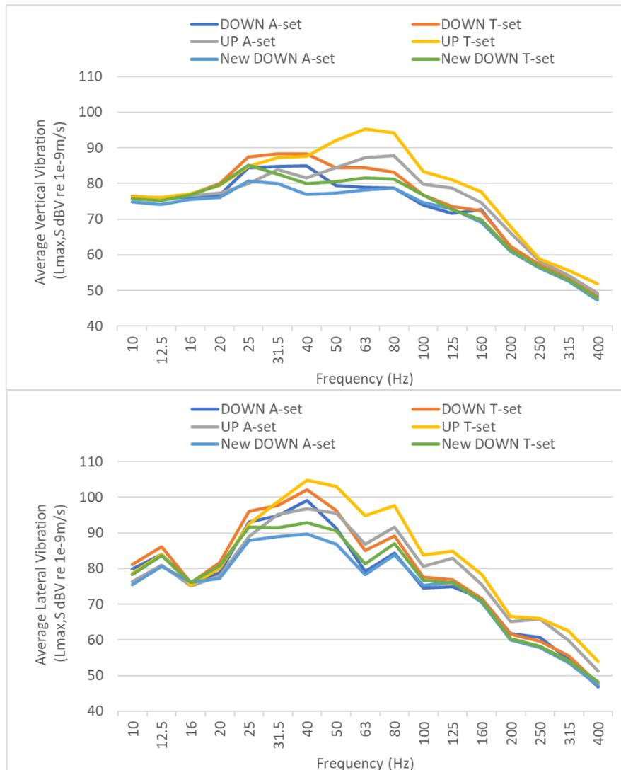
Figure 5: Arithmetic average vibration spectrum by axis, track and train type
