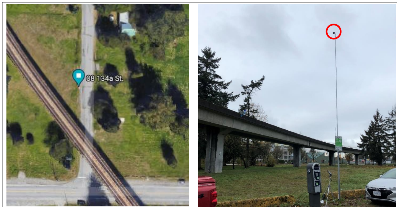
Figure 3: Example noise measurement configuration (Location 8) with microphone circled in red
