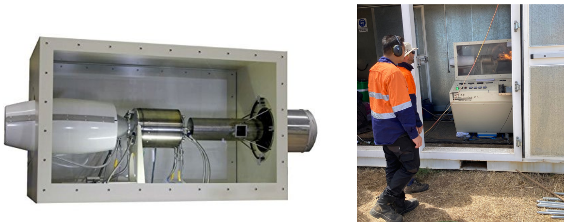
Figure 3: Close up image of the SR-30 turbojet engine, showing the inlet HushKit, turbine and exhaust inlet (left); photograph of turbojet engine in the acoustically treated shipping container on startup (right).
