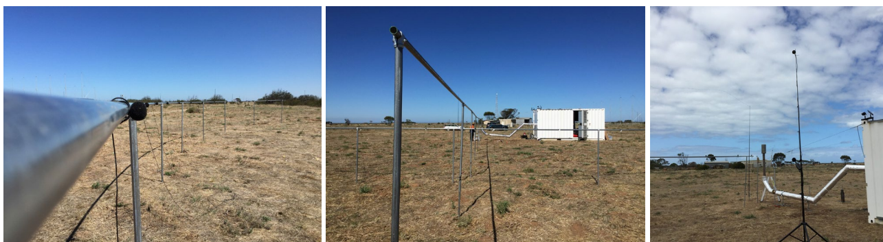
Figure 4: Photographs of the “upwind” circular arc array (left); the “downwind” logarithmic line array (and “downwind” circular arc array) with the shipping container in the background (middle); the roving SLM with lower and upper microphones, the windsock streamer and the exhaust outlet and shipping container (right).
