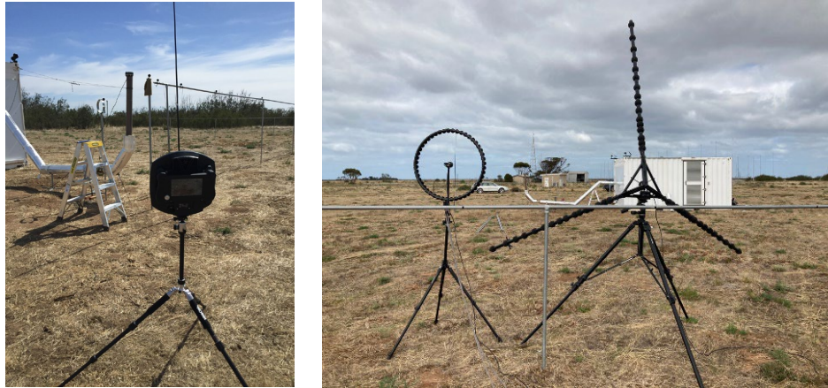
Figure 5: Photographs of the acoustic cameras used to visualise the sound field. Left-hand image is the portable SoundCam (kindly supplied by Resonate Consultants) with compression driver on the stack; and the right-hand image shows the gfai tech Ring48 and Star48 acoustic cameras (kindly supplied by HW Technologies).
