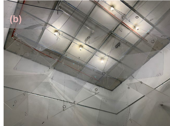
Figure 1: Geometry of the UTS reverberation room. (a) Dimensions, where HT means the height of the wall from floor level, with the default units being millimetre. (b) Suspended diffusers in the reverberation room.
