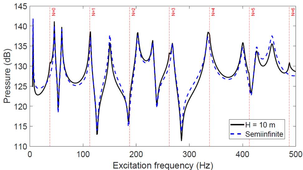
Figure 1: Acoustic pressure at an observation point of  $(a/2, b/2, 5)$  for a plate in a heavy fluid domain with a far free surface ( $H = 10$  m), and in a semiinfinite fluid domain
