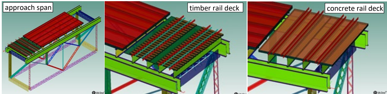
Figure 6: SEA models of the bridge (9 m long segment of approach span)
