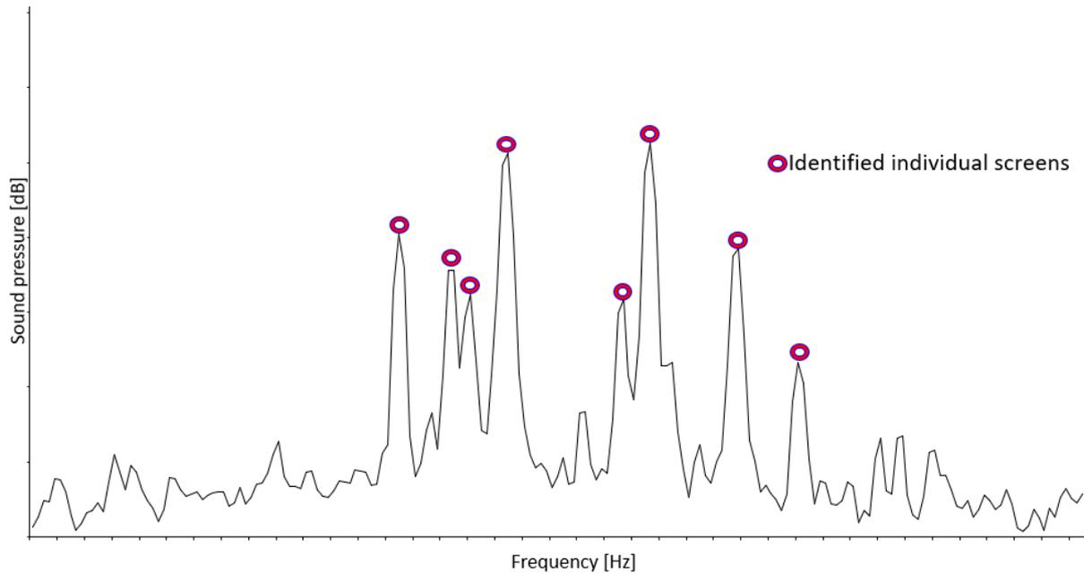
Figure 3: Identification of the runspeed of individual vibrating screens by narrowband FFT analysis.
