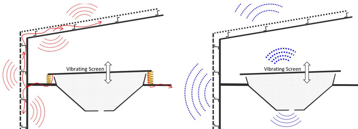
Figure 2: Low frequency sound mechanisms (left: structure-borne, right: airborne).
