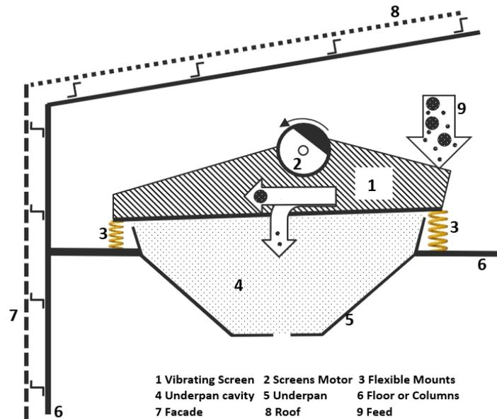
Figure 1: Basic schematic identifying parts.
