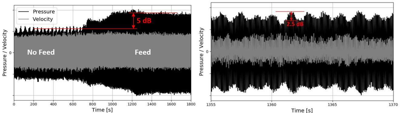
Figure 4: Processing plant sound pressure (black) and facade vibration velocities (grey).
