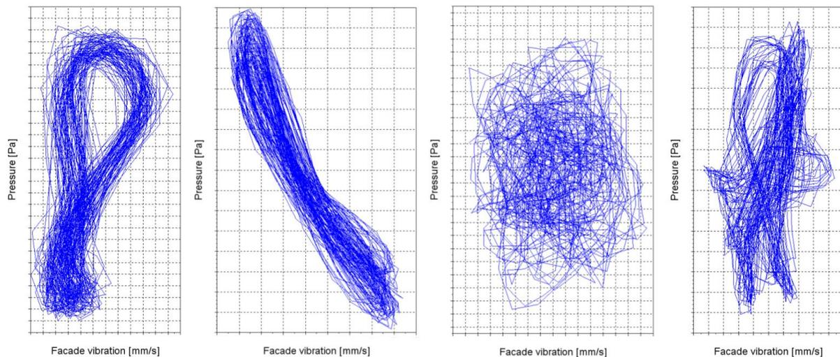
Figure 5: Example phase relationships between pressure and facade vibration measured in an airborne dominant environment.
