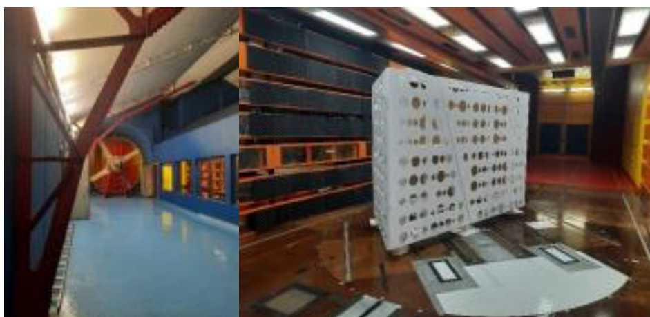
Figure 9: Scale prototype panel in wind tunnel (Cnam, Institut Aérotechnique)
