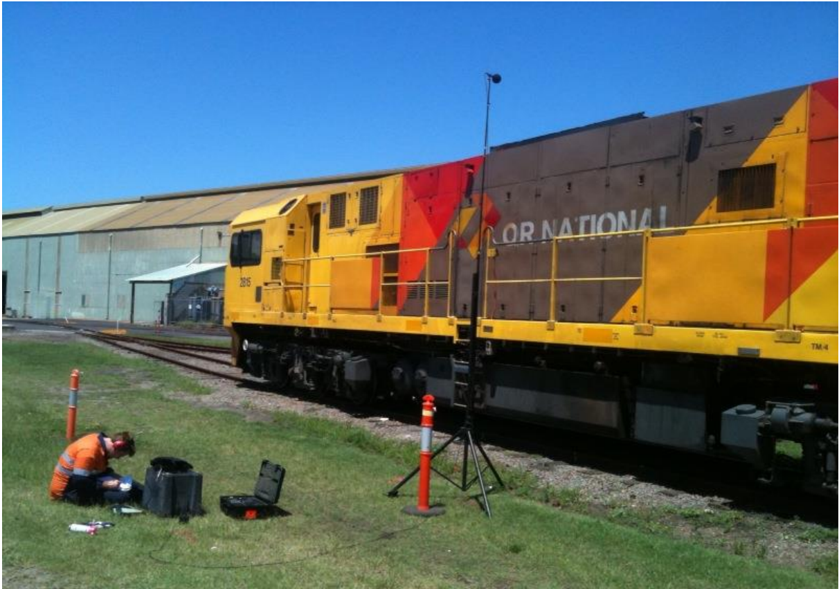
Figure 2 – Muffler noise testing at 3m from exhaust outlet
