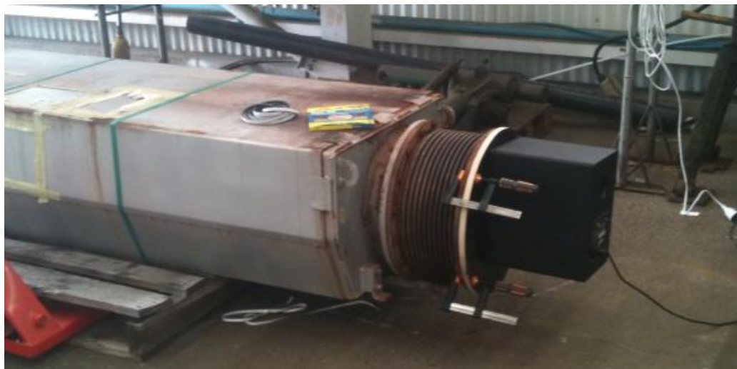
Figure 3 – Full scale cold testing of original muffler using a pink noise source
