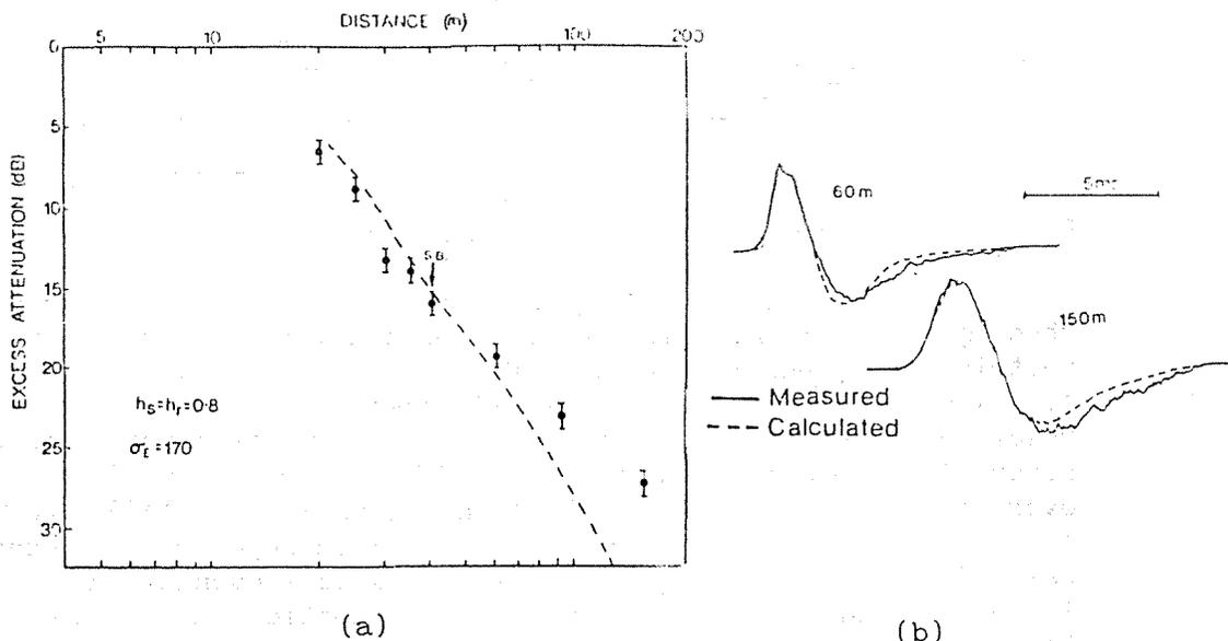
Fig. 7 (a) Experimental results and --- creeping wave prediction. (b) Comparison of measured and calculated pulse shapes.
