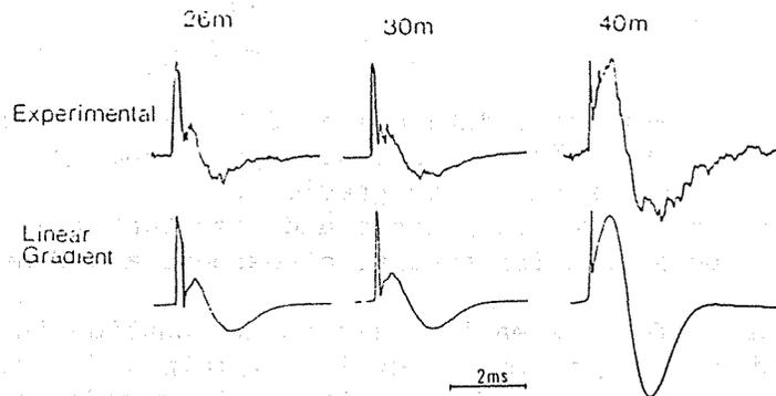
Fig. 4 Comparison of measured and calculated pulse shapes.
