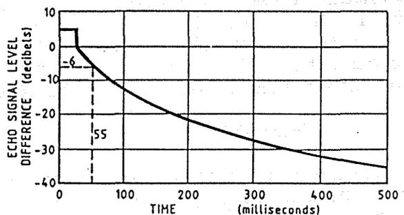
Fig. 2. RELATIONSHIP BETWEEN LEVEL OF REFLECTED SOUND AND TRANSIT TIME TO AVOID ANNOYING "ECHOES".
