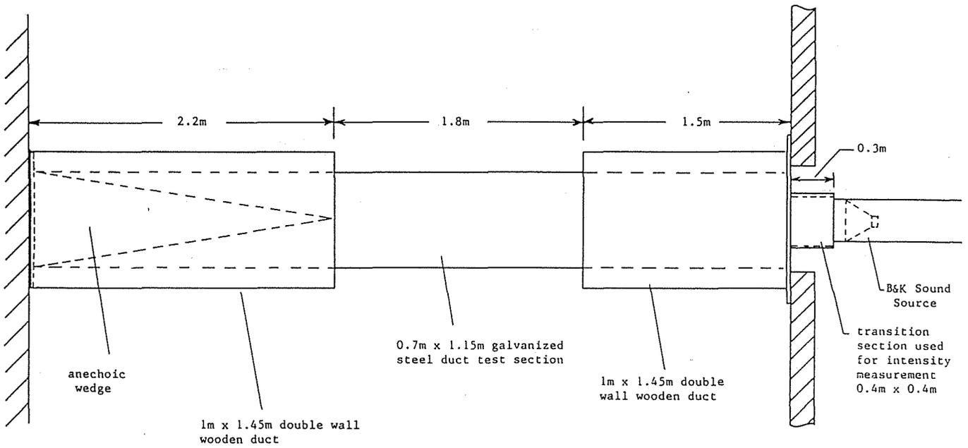
Figure 1. Experimental arrangement.
