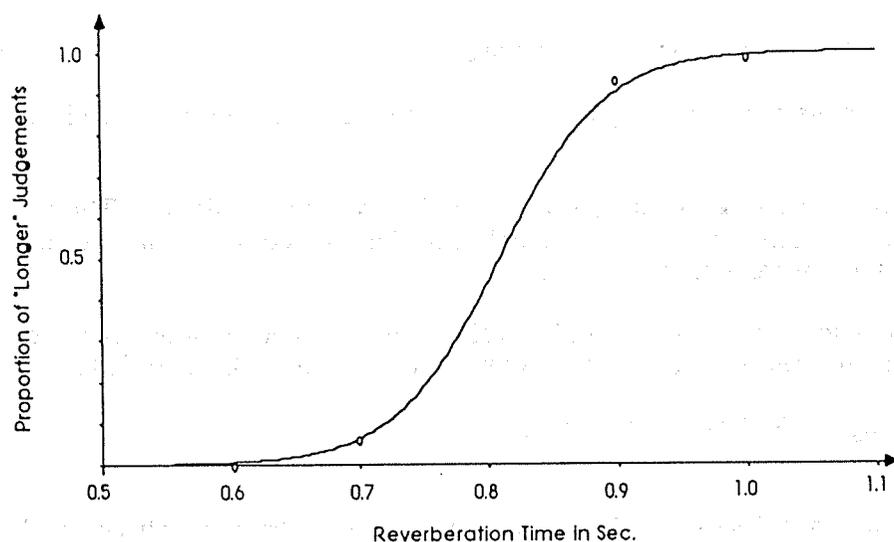
**Fig. 4.2.1** The measured data and psychometric function obtained by regression (average of three subjects) for a standard reverberation time of 0.8 s at 2 KHz
