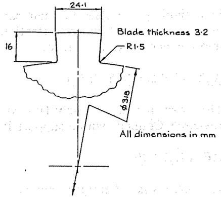
Fig. 2.2: Rotating Blade Single Tooth Model Dimensions
