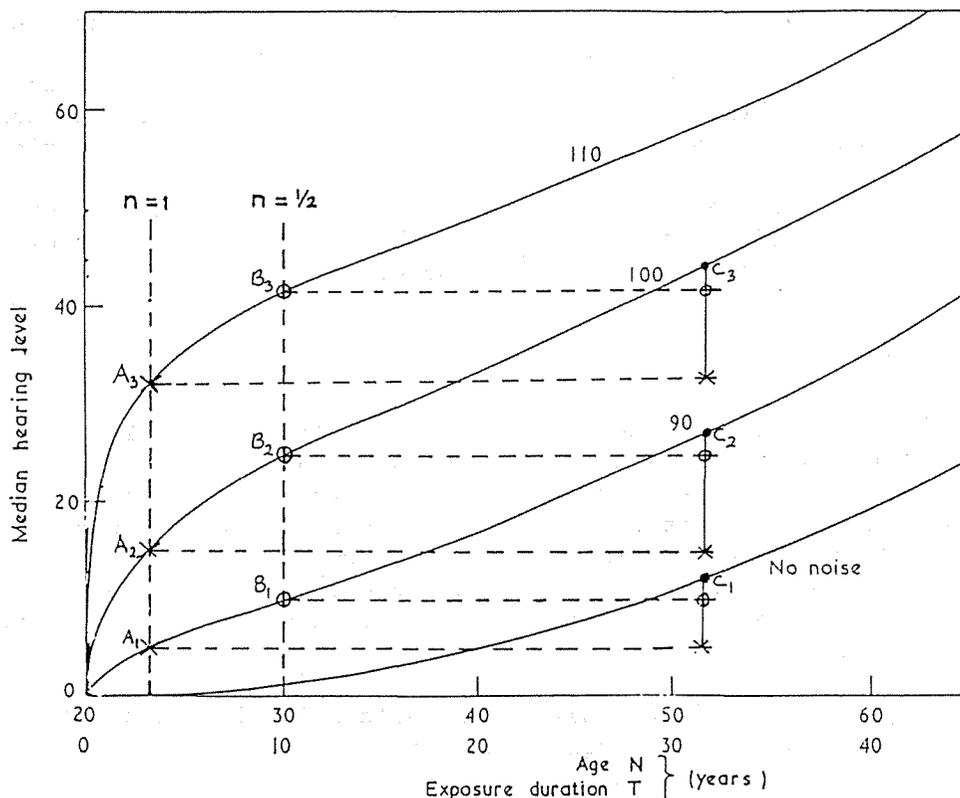
Figure 1. Illustration of the better fit of the 6 dB ( $n=1/2$ ) rule over the 3 dB ( $n=1$ ) rule for Burns and Robinson's data [4].
