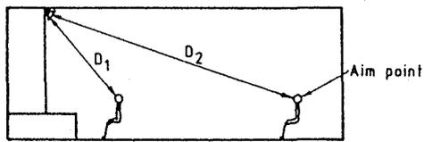
Fig. 6. BASIS FOR INITIAL LOUDSPEAKER POSITIONING ( $D_2/D_1 \leq 3$ )
