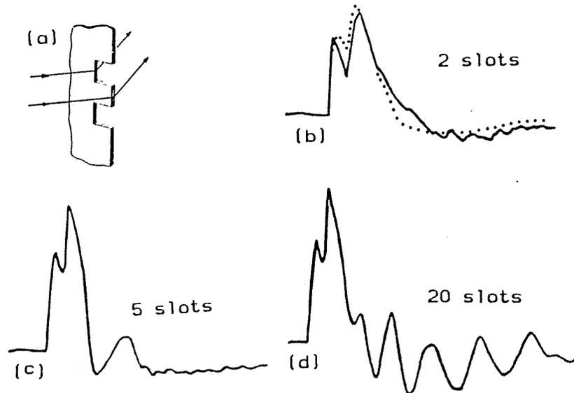
Fig.6: Geometry and waveforms from castellated diffraction.
