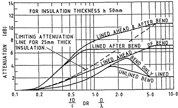
Fig. 7. APPROXIMATE ATTENUATION OF LINED AND UNLINED MITRE BENDS WITH SHORT CHORD TURNING VANES.
