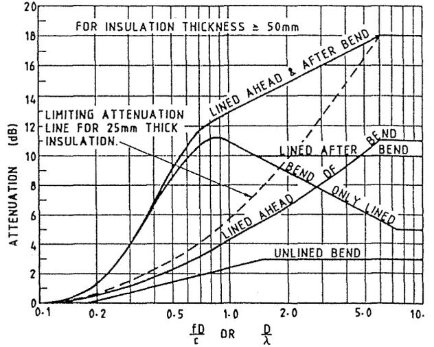
Fig. 6. APPROXIMATE ATTENUATION OF LINED AND UNLINED SHORT RADIUS BENDS ( $R/D \leq 1.0$ ).
