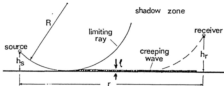
Fig.6 Formation of a shadow zone in a linear sound speed gradient.
