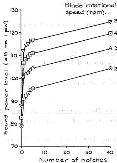
Fig. 3.2: Effect of Gullet Number and Rotational Speed on Sound Power Radiated
