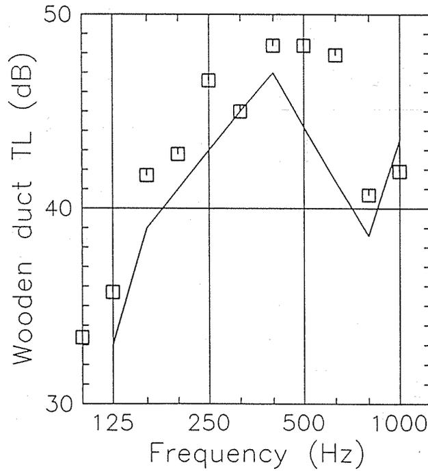
Figure 6. TL data for double wall wooden ductwork used to terminate and connect the test section to the sound source.
