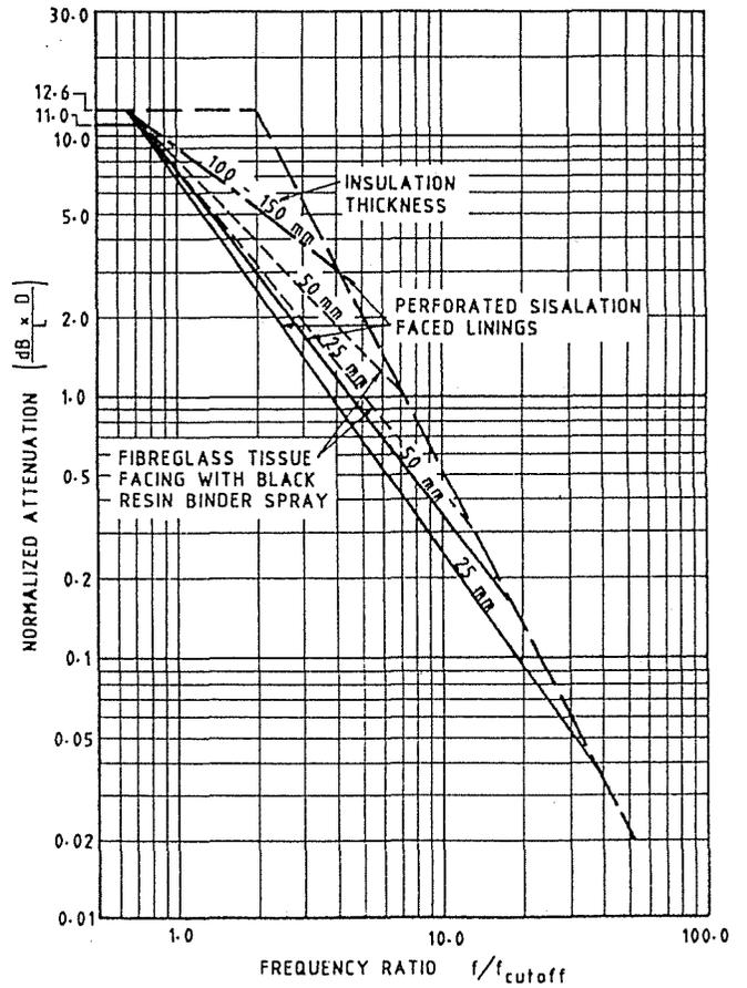
Fig. 4. NORMALIZED ATTENUATIONS AT FREQUENCIES NEAR AND ABOVE THE CUTOFF FREQUENCY.
