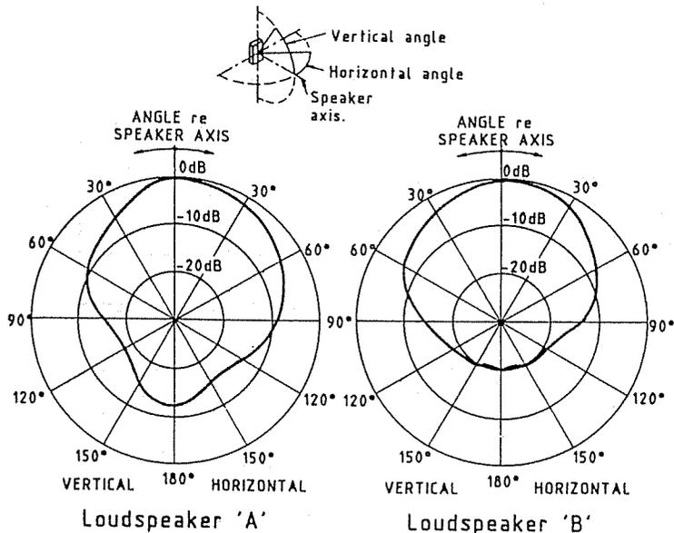
Fig. 3. TYPICAL DIRECTIVITY PATTERNS FOR TWO LOUDSPEAKERS HAVING ABOUT 100 WATTS CAPACITY.
