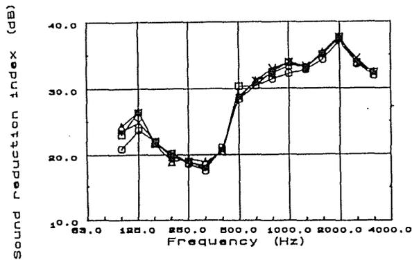
Figure 5 Sound reduction index obtained in various ways using the intensity technique.
