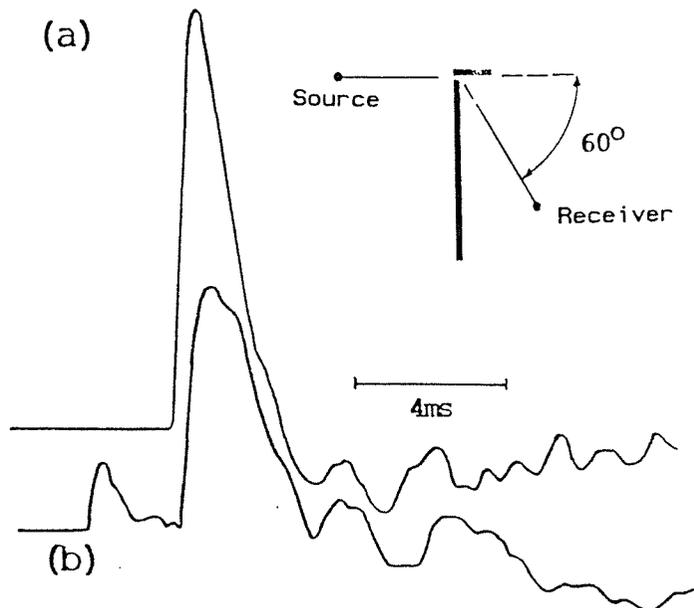
Fig.7: Effect of a crack: (a) diffraction around sealed corner, (b) is with crack present, showing pre-pulse.
