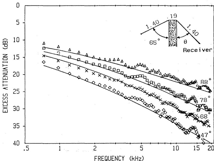
Fig.5: Results for a thick barrier compared with predictions of Pierce.
