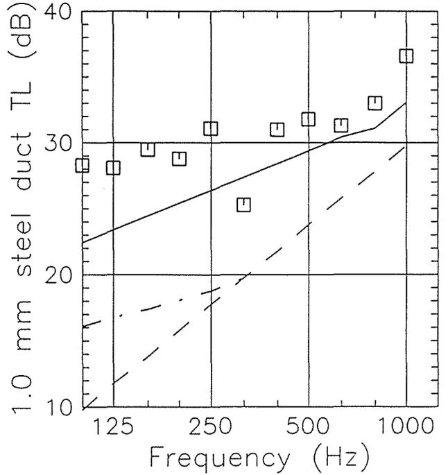
Figure 3. TL data for a steel duct of 1.15 x 0.7m cross section and 1.0mm wall thickness.
