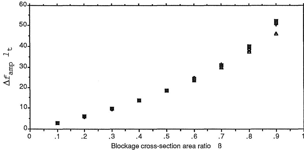
Fig.2 Weighted amplitude of eigenfrequency shifts as function of  $\beta$
