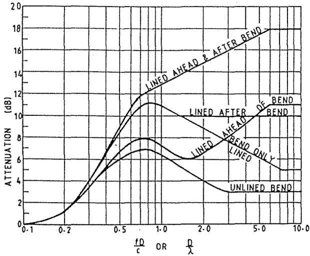
Fig. 5. APPROXIMATE ATTENUATION OF LINED AND UNLINED MITRE BENDS WITHOUT TURNING VANES.
