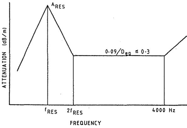
Fig. 1. ATTENUATION OF BARE RECTANGULAR STEEL DUCTS.
