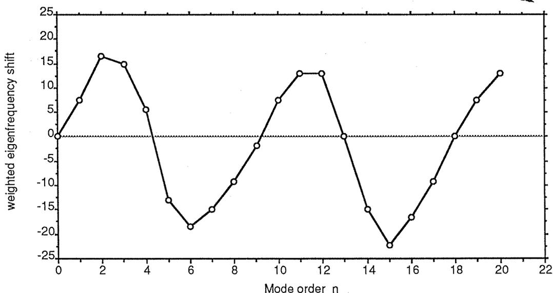
Fig.3 Measured eigenfrequency shift pattern of a rectangular blockage.
