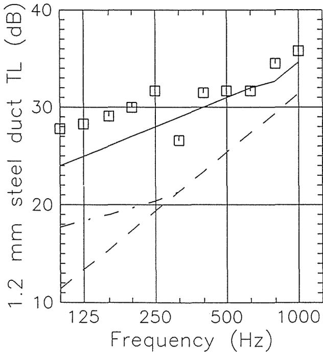
Figure 2. TL data for a steel duct of 1.15 x 0.7m cross section and 1.2mm wall thickness.
