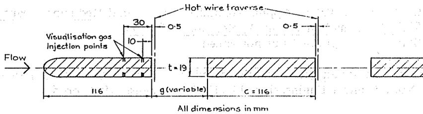
Fig. 2.3: Cross-section of Array of Model Saw Teeth in Wind-tunnel
