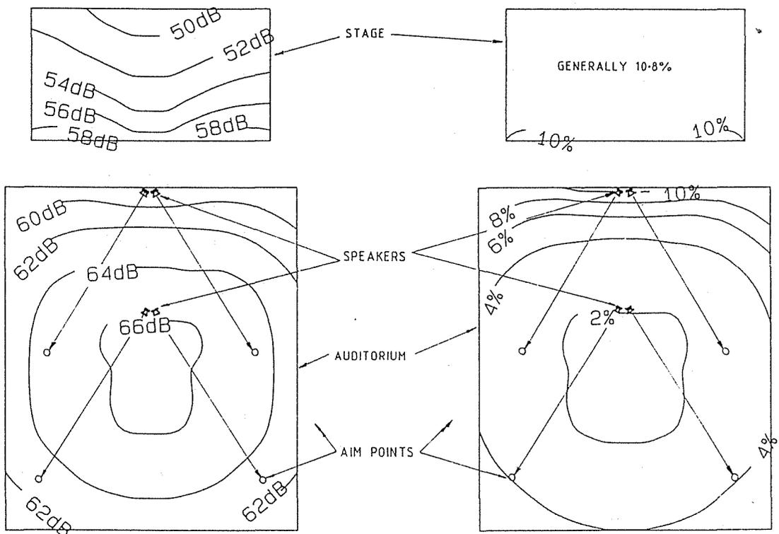
Fig. 8. DIRECT SOUND LEVELS AND PERCENTAGE ARTICULATION LOSSES FOR A TYPICAL HIGH SCHOOL AUDITORIUM WITH 4 x 100 WATT SPEAKERS AND 40dB(A) BACKGROUND LEVEL. (S/N ratio  $\geq 25$  dB)
