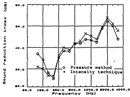
Figure 1 Sound reduction index of the facade, i.e. windows, open air intake and wall measured in different ways.
