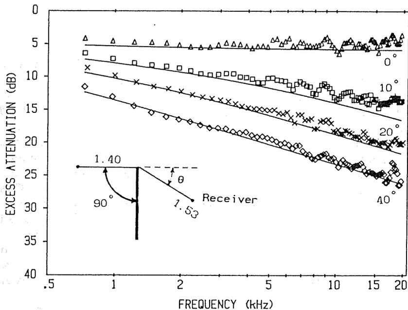
Fig.4: Frequency dependence of excess attenuation compared with prediction of Hadden and Pierce.
