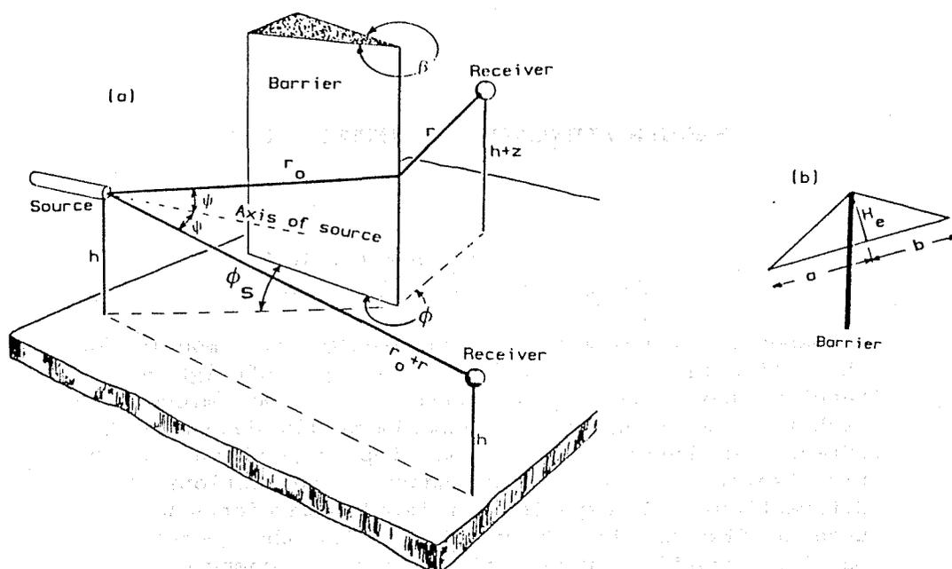
Fig.1: The measurement geometry.
