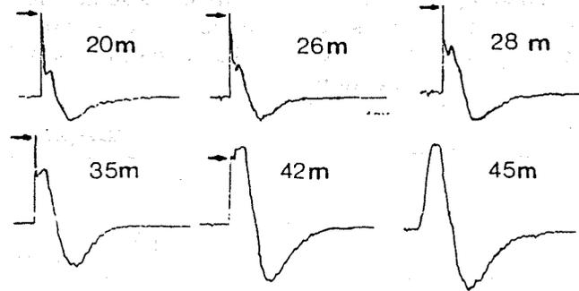
Fig. 3 Impulse waveforms measured at various distances from the source.
