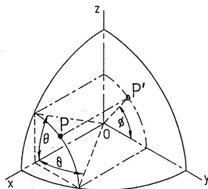
Fig. 4. DEFINITIONS OF ANGLES  $\theta$ ,  $\phi$  FOR LOUDSPEAKER DIRECTIVITY TOWARDS P RELATIVE TO MAIN SPEAKER AXIS.  $\theta$  IS AN ANGLE IN THE x-z AND x-y PLANES. P' IS PROJECTION OF P ONTO y-z PLANE AND  $\phi$  IS IN y-z PLANE. (O-x = Main speaker axis)
