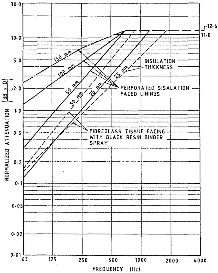
Fig. 3. NORMALIZED ATTENUATIONS AT FREQUENCIES WELL BELOW THE CUTOFF FREQUENCY.
