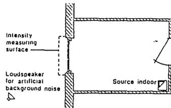
Figure 3 Sketch showing the principles of measuring sound reduction index with a noise source indoors. Plan view.
