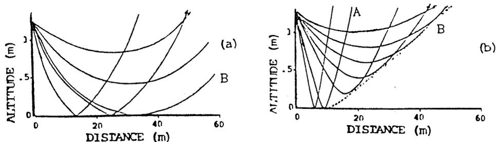
Fig. 1 Ray paths in (a) linear gradient and (b) a non-linear gradient.
