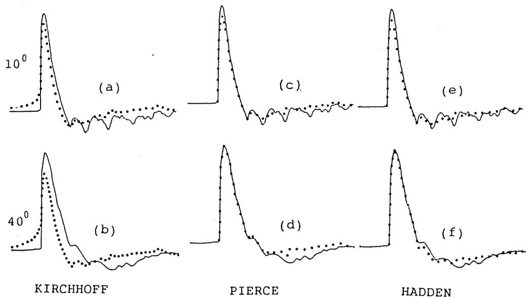
Fig.2: Experimental (solid) and theoretical (dotted) waveforms for the geometry in Fig.4.
