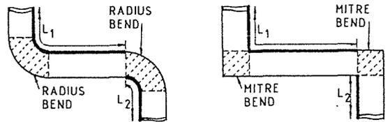
Fig. 8. SCHEMATIC ILLUSTRATION OF HOW TO MEASURE LENGTHS OF LINED DUCT SEGMENTS INCLUDING BENDS. HEAVY LINES INDICATE LENGTHS TO BE INCLUDED IN MEASUREMENT.
