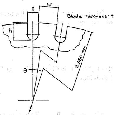
Fig. 2.1: Rotating Blade Model Tooth Geometry
