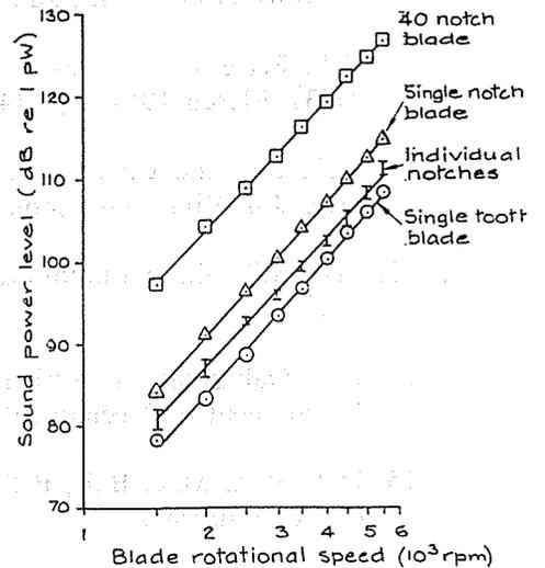
Fig. 3.3: Effect of Blade Configuration and Rotational Speed on Sound Power Radiated
