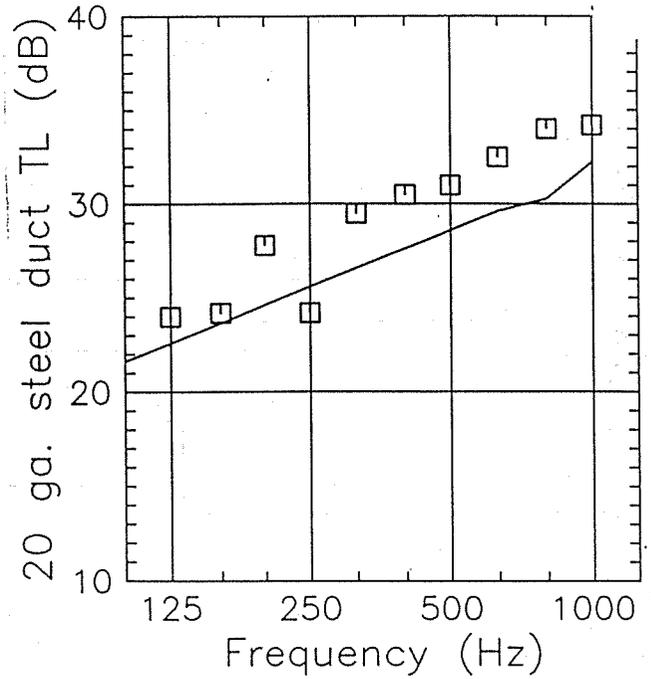
Figure 4. TL data for a steel duct of 1.15 x 0.7m cross section and 0.8mm wall thickness.
