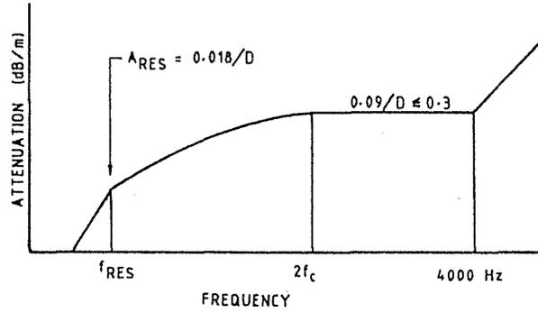
Fig. 2. ATTENUATION OF CIRCULAR STEEL DUCTS OR HEAVY RECTANGULAR DUCTS.
