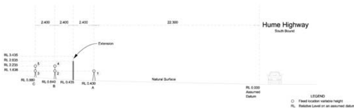
Figure 4: Cross section showing microphone positions A, B & C and barrier position
