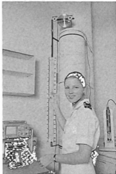
Figure 1. Midshipman Michele Miller monitors the pulse signals of a commercial echo-sounder whose transducer is mounted in a vertical tube of water.
