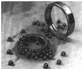
Figure 1. A Damaged Rolling Element Bearing
