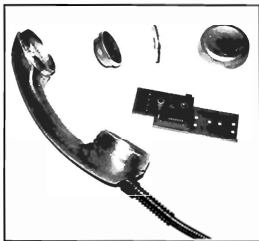
Fig. 5 Hearing Aid Coupling Coil and Amplifier for Public Telephones
