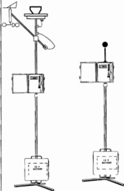
Battery operated loggers incorporating software to down-load data into your computer. Completely weather-proof and rugged
