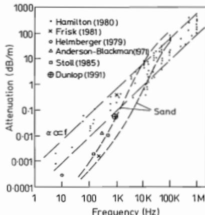
Figure 3. Laboratory and field data of sediment attenuation constant plotted against frequency. Also shown are curves of the calculated attenuations of two sand samples based on Biot theory (from Stoll [29]).
