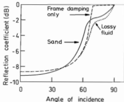
Figure 4. Relationships between the reflection coefficient and angle of incidence of an acoustic wave incident on a water sediment interface calculated by applying Biot theory to a sand sediment, the sand sediment with frame damping only, and a lossy fluid of the same approximate damping constant (from Dunlop [6]).
