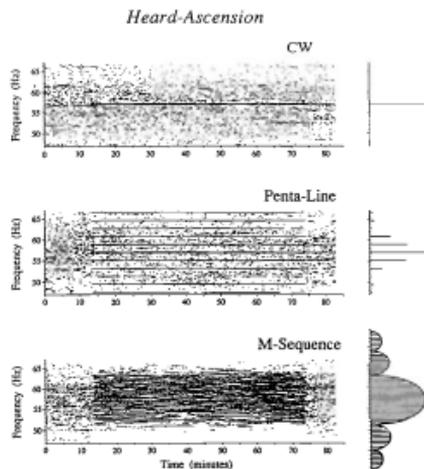
Figure 4. An hour-long example of each type of signal as received at Ascension Island. To the right is the spectrum of each transmitted signal.
