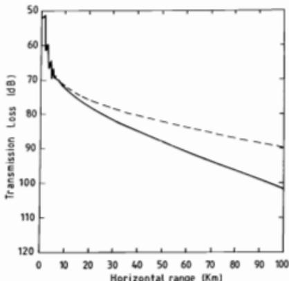
Figure 2. Transmission Loss at frequency 10 Hz in water of depth 200 m over a coarse quartz sand seabed. Key: as for Fig. 1
