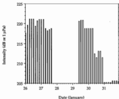
Figure 2. Timing and intensity of the HIFT transmissions. There was a 39 hour period of silence centred on January 28 while repairs were made to the acoustic source array.
