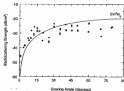
Figure 5. Bottom backscattering strength, frequency 100 kHz, shallow site W1, frame measurement.
