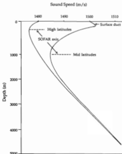
Figure 1. Generalised vertical profile of sound speed in the ocean. Acoustic thermometry takes advantage of the deep sound (SOFAR) channel axis.
