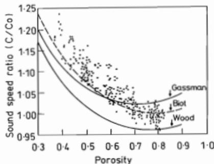
Figure 1. Measured values of sound speed ratio ( $c/c_0$ ) plotted against sediment porosity (from Hamilton [7]). Also shown are the theoretical curves of Wood, Gassman using a frame modulus of 400 MPa, and Biot using a frame modulus of 40 MPa.
