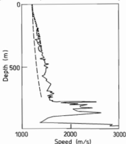
Figure 2. Relationship between sound speed and depth of sediment for an ooze-chalk-limestone sequence - solid curve from field data, dashed and dotted curves as predicted from Biot theory with different estimates of porosity (from Ogushwitz [18]).
