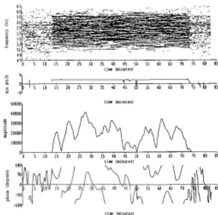
Figure 5. Detail of a one-hour's reception of an M-sequence signal at Ascension Island. The bin shift (1 unit = 0.0139 Hz) represents the Doppler shift due to source-ship motion.
