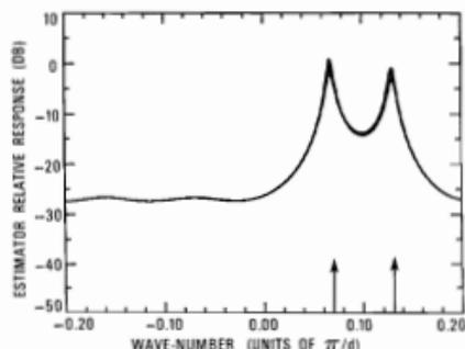
Figure 2. Response from sector focussing stability (SFS) technique using eigenvectors 3-6 showing limited spread of results from different simulations and robustness to phase errors (from Ref. 4).
