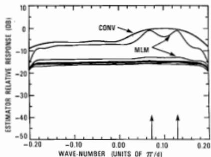
Figure 1. Relative responses for conventional (CBF) and adaptive (MLM) beamformers (from Ref. 4). The top curve shows the conventional estimator response, with and without phase errors (no discernible difference), the next curve shows the response from the MLM for the no-phase-error case, and the bottom five curves are the MLM responses for independent simulations with 5° phase errors.
