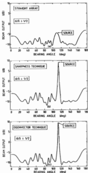
Figure 3. Variation of the output power with beamsteer angle for an adaptive beamformer processing real data from an experimental towed array: (a) assuming that the array is straight, (b) using the array shape inferred from the sharpness optimisation technique, and (c) using the hydrophone positions estimated by the eigenvector technique. The frequency of interest is close to the design frequency (i.e.,  $d = \lambda/2$ ) of the array (from Ref. 11).
