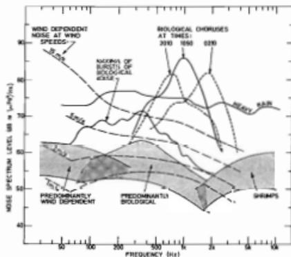
Figure 1. Summary of the components of ambient noise in shallow water in the Timor Sea. The shaded areas indicate the prevailing noise at low wind speeds. The wind dependent noise curves were determined from measurements at many locations around Australia (ref. 22).
