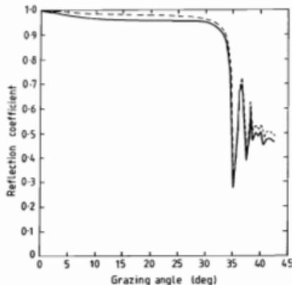
Figure 1. Reflectivity vs Grazing angle of a coarse quartz sand at frequency 10 Hz. Key: ——— Coupling between P and SV waves included; - - - - P-SV Coupling neglected.
